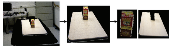
Figure 3: Illustration of the preprocessing pipeline. Left: input point cloud; Middle: point cloud after passthrough filtering; Right: segmented candidate object and removed table surface.
